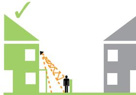
4. Direct lights downwards. If uplighting has to be used, install hoods or shields above the light, to reduce the amount of wasted upward light.
