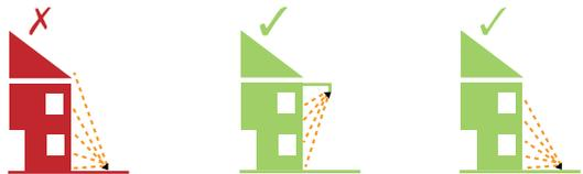
5. Do not install equipment that spreads light above the horizontal.
