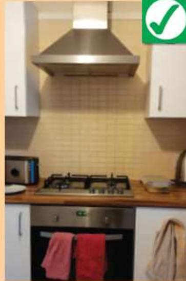
This layout meets the minimum requirements as there is adequate worktop to both sides of the cooker and suitably located extraction.
