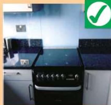
This cooker location meets the minimum requirements for a suitably sited cooker with sufficient worktop to both sides of it.
